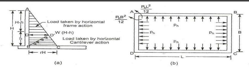
Fig. 13.6 Pressure Diagram
